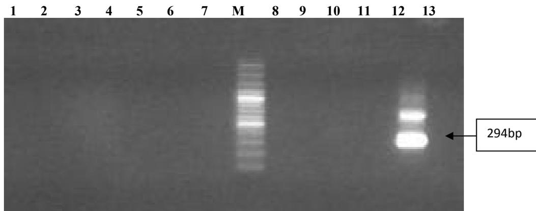
**Fig. 4: *T. congolense* Kilifi positive control K45 DNA amplified with TCK 1 and TCK 2 primers.** Test samples labelled 1–11; 13-negative control (-v) and 12 is K45 positive control, 100 base pair ladders labelled 'M'. The reference DNA has been amplified with a product size of 294 bp.
